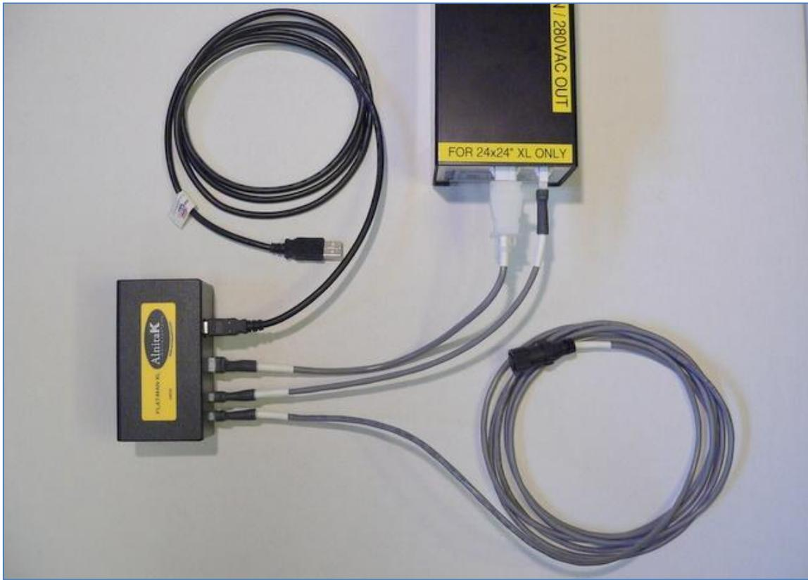
2. Plug the Flat-Man XL controller output cable into the HV power supply 6-position connector.
