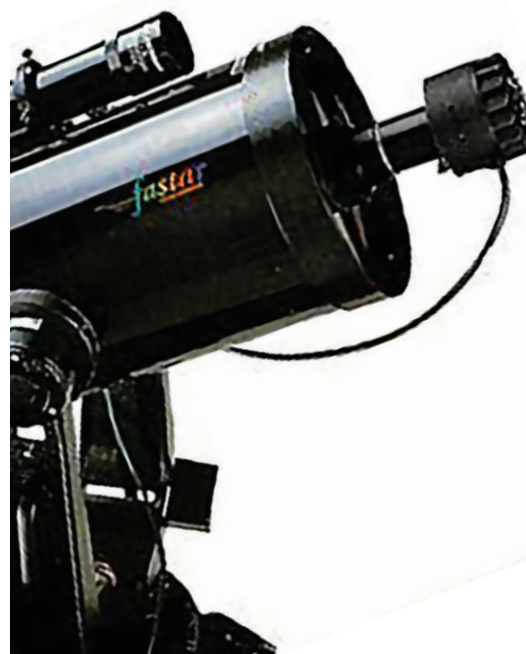
Fig. 6: The 8-inch f/2 Fastar carried a PixCel CCD camera ahead of the corrector plate. In a fast telescope, it turns out that the best place for a compact image sensor is at the prime focus.
