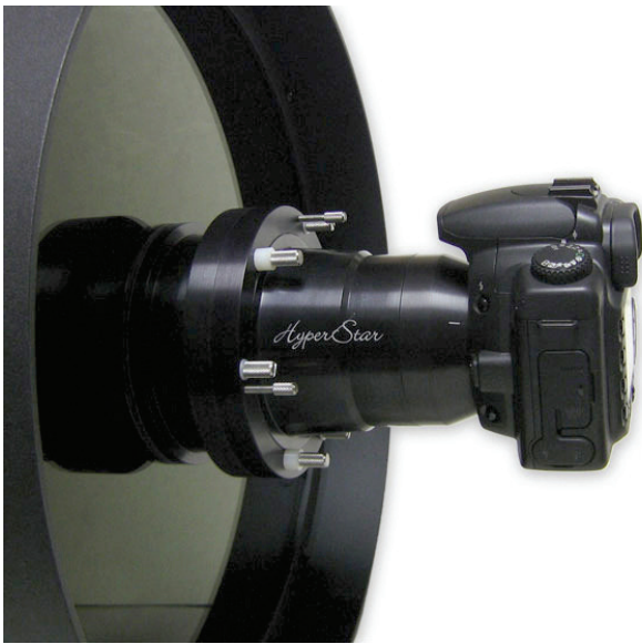
Fig. 7: The Starizona HyperStar worked extremely well with APS-C DSLR cameras. By combining fast optics, short focal length, and wide field, it paved the way for the Rowe-Ackermann Schmidt Astrograph.
