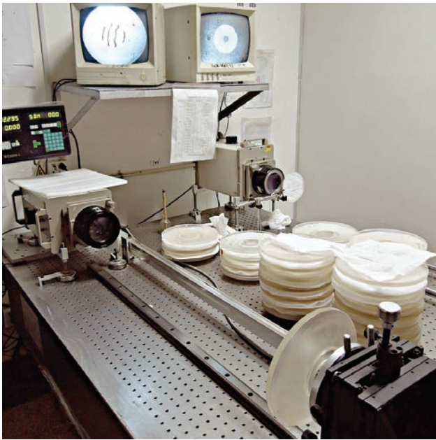
Fig. 15: All RASA primary mirrors are tested on an optical bench by means of laser interferometry. In the picture, stacks of polished primary mirrors await testing.
