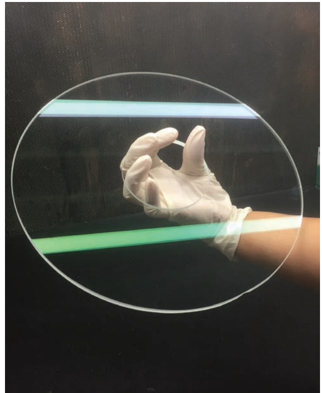
Fig. 11: The Schmidt corrector plate is not a simple optical window, it is actually an aspheric lens. Celestron's founder, Tom Johnson, revolutionized the manufacture of this optical element with his patented process, and the Schmidt corrector in the RASA is made in this same way.
