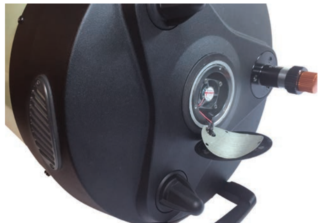
Fig. 14: The 12VDC MagLev fan along with improved venting allows for good airflow within the optical tube. This helps cool the telescope to ambient temperature.
