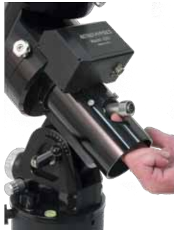
2. Work control box cable end out through R.A. Cable Access Hole
